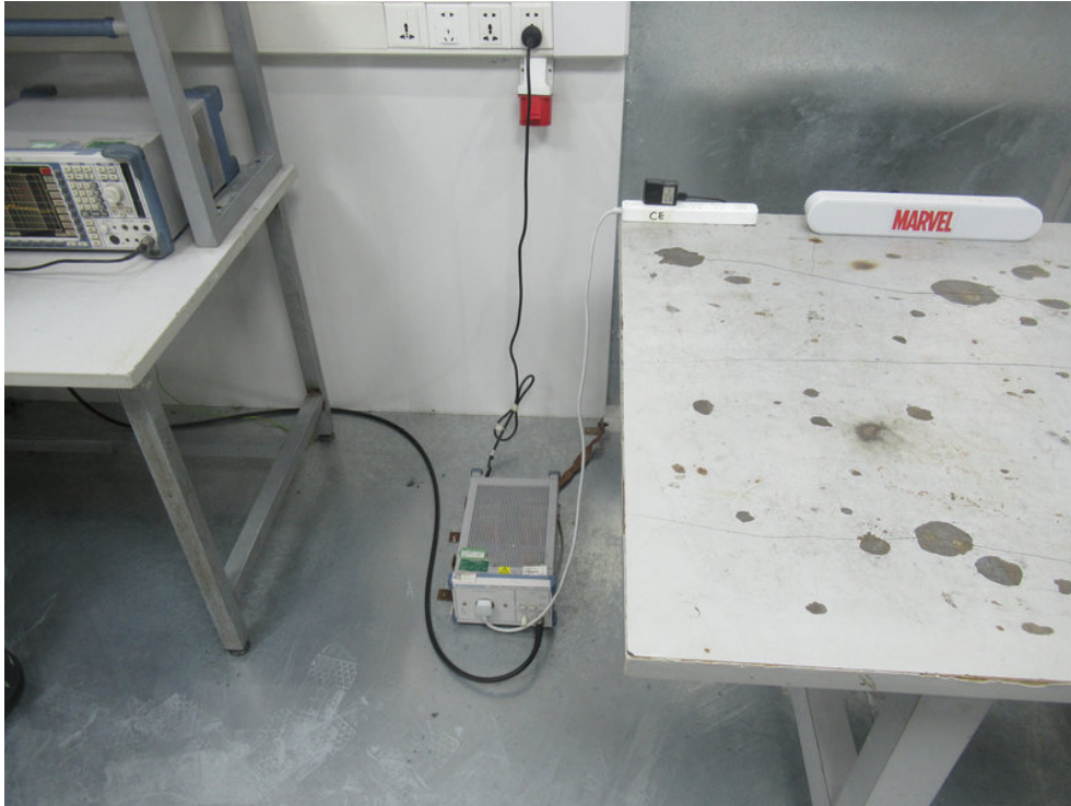
Photo of Conducted Emission Measurement
