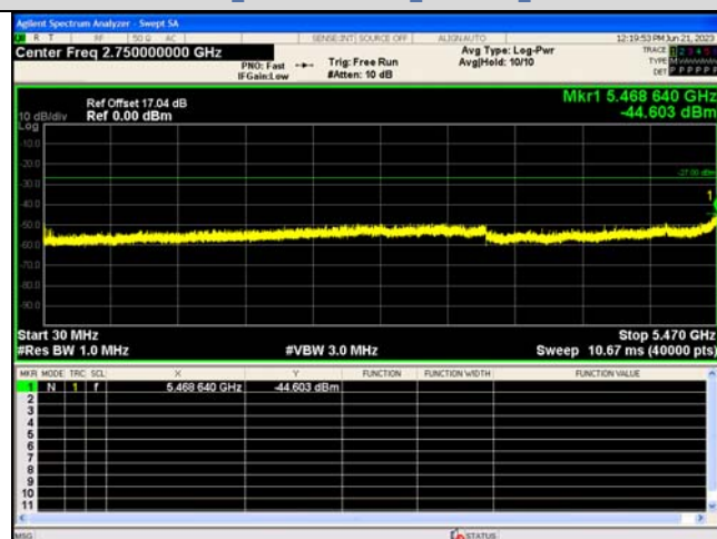
Spurious Emission:30.0~5470 MHz IEEE 802.11n_Channel 140_20MHz_Antenna 0
