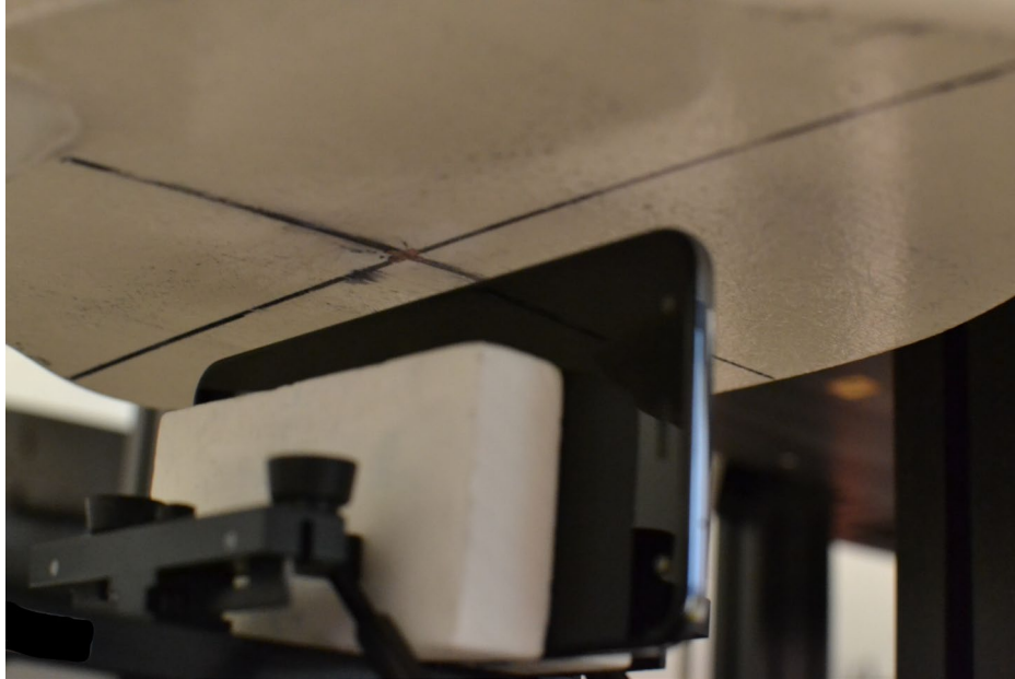
SAR Test Setup Photo 16 – Left Edge 10mm
