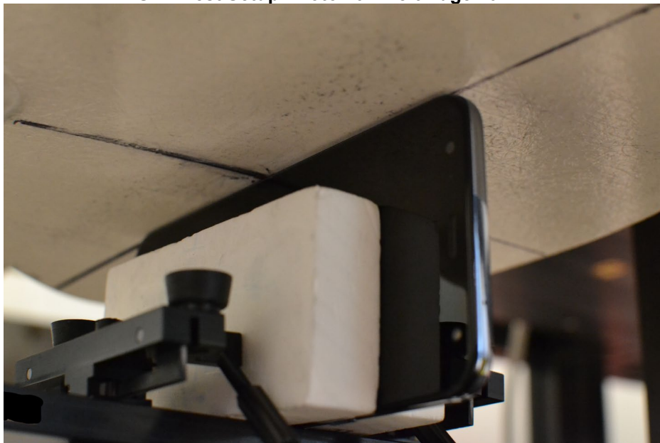
SAR Test Setup Photo 17 – Left Edge 0mm
