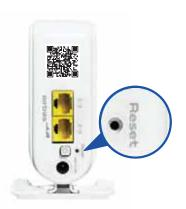
To return the device to factory settings, press down on the reset button (in the small opening on the back shown above) for 5 seconds and release. A metal paperclip (with an extended tip) or strong toothpick are typically good choices for this task. When the reset process is triggered, the LED in the front will "blink rapidly" and the device will reboot to factory settings.
