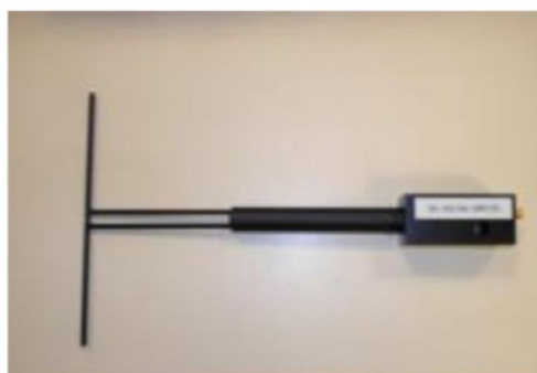
Figure 1 – Satimo COMOSAR Validation Dipole
