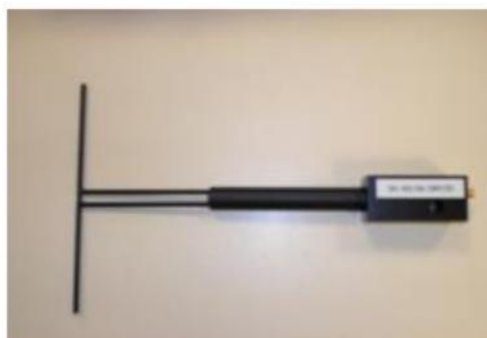
Figure 1 – Satimo COMOSAR Validation Dipole
