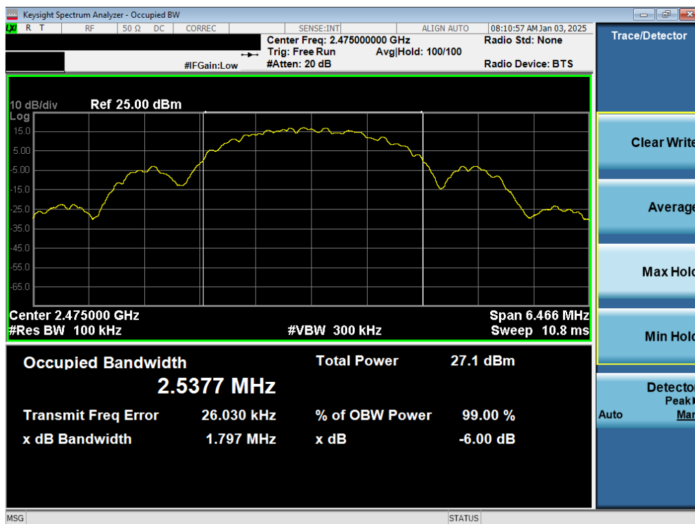
Plot 7-3. 6dB BW & 99% OBW Antenna WF8 (802.15.4, Ch. 25)
