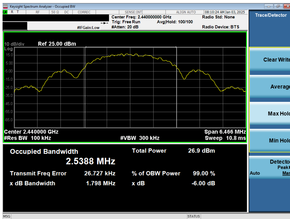
Plot 7-2. 6dB BW & 99% OBW Antenna WF8 (802.15.4, Ch. 18)
