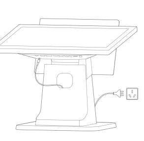
Put the power cable through the cable hole on the prop back; Turn the display upward to find the cable hole on the front side of the prop; Plug the power adapter into the power port on the back of the display; Plug the other side of the adapter into the AC socket. • Please plug the AC power plug into the AC socket which complies to the input marked on the power adapter of the accessory;
