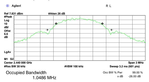
Transmit Freq Error -11.611 kHz x dB Bandwidth 1.331 MHz
