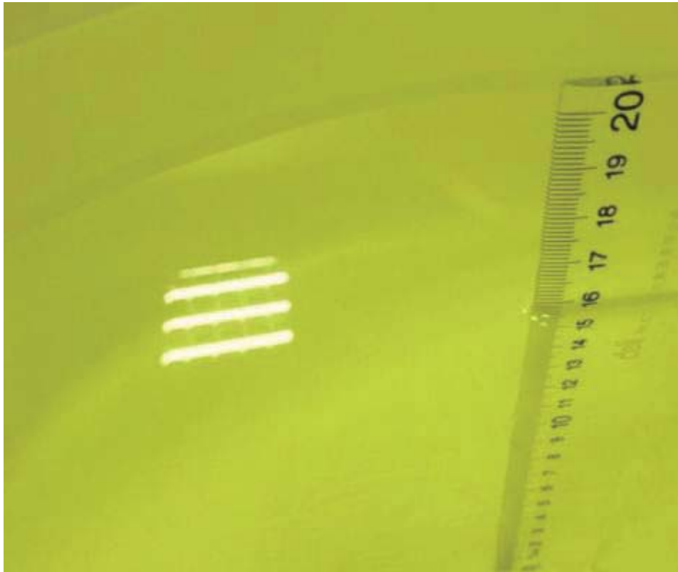
Picture9-3:Liquid depth in the Flat Phantom (1800/1900 MHz Head)
