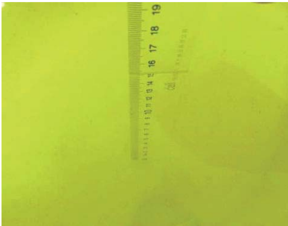
Picture 9-4: Liquid depth in the Flat Phantom (2450 MHz Head)
