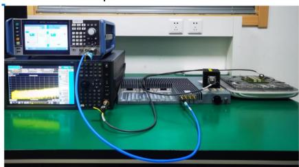
Radiated Spurious Emissions (30MHz-1GHz)
