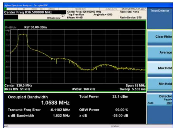
LTE Band 26 16QAM 15MHz CH-High
