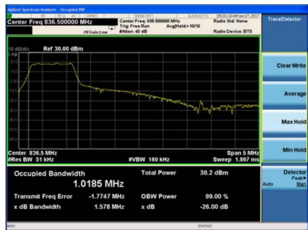
LTE Band 26 16QAM 5MHz CH-High
