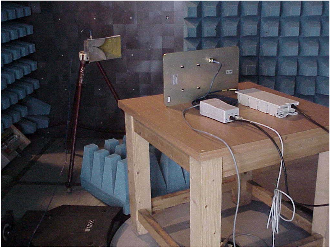
RE 1-26 GHz test set-up detail
