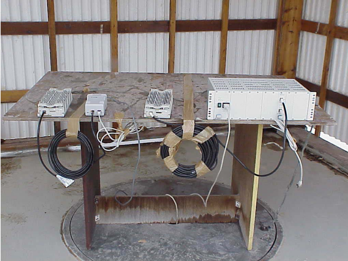
Set-up, system digital radiated emissions test 30 - 1000 MHz
