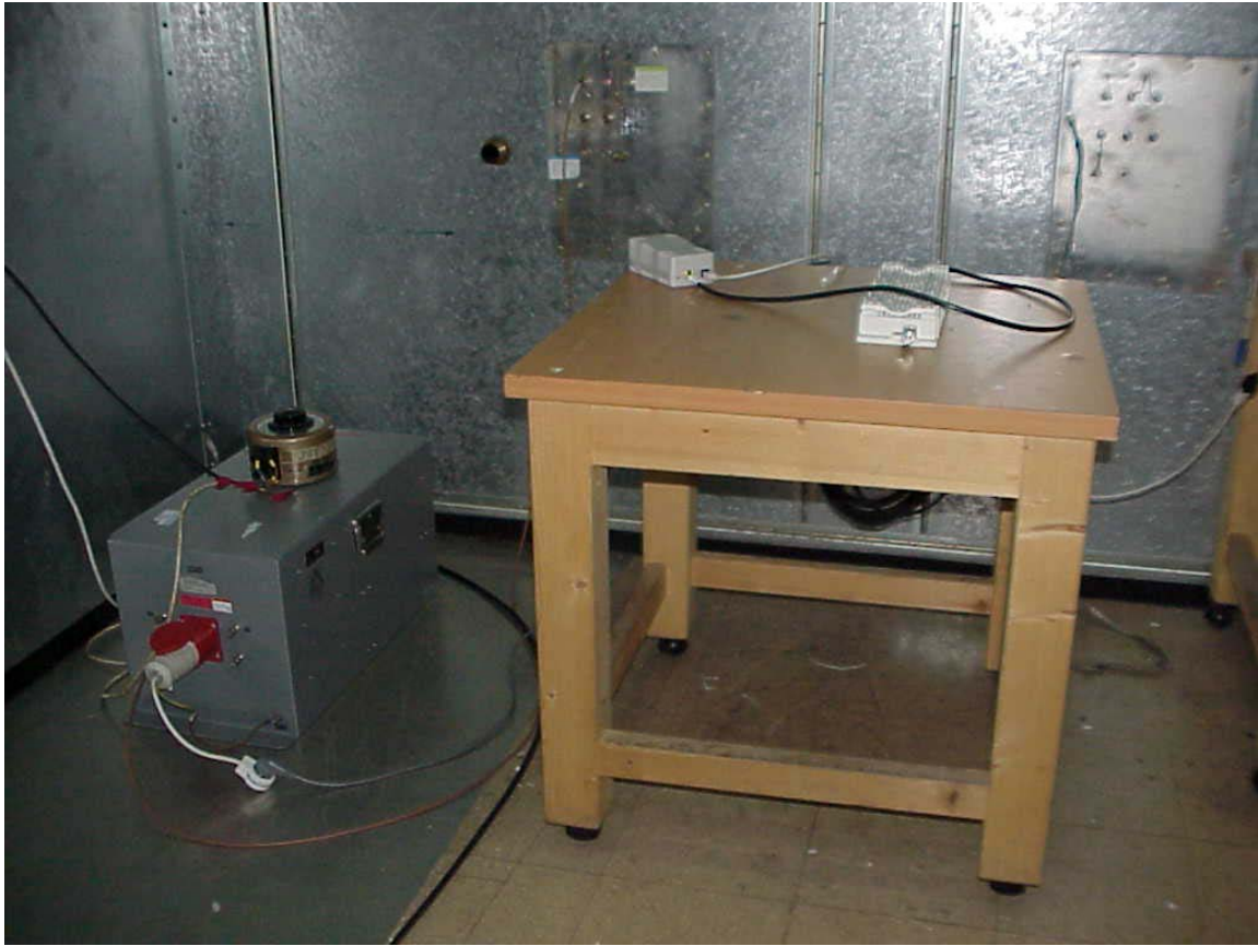
AC line conducted emissions test set-up
