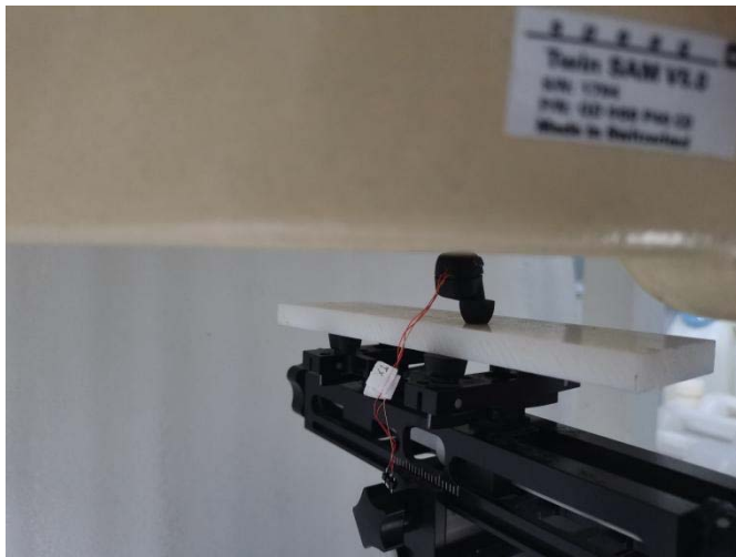
Fig-4.1 Front of EUT with 0 cm Gap (Head Mode)
