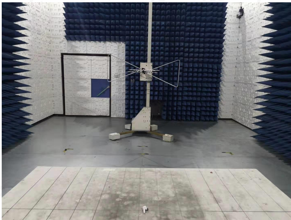
RADIATED EMISSION TEST SETUP ABOVE 1GHZ
