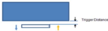
Picture : Proximity sensor triggering distances assessment (Back side)
