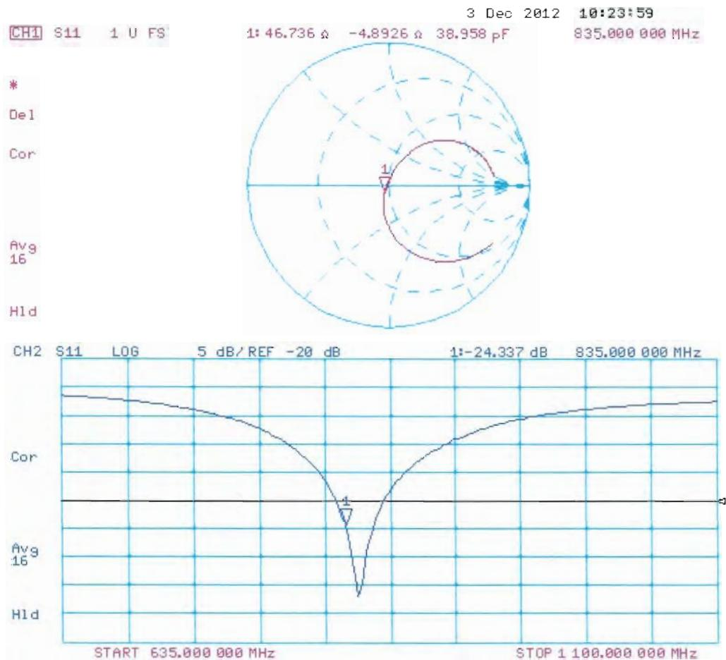
Dipole D835V2 – SN: 480 Antenna Parameters measured: 2014-01-31.
