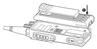
2. Press and push the battery into the battery slot until a click is heard.
