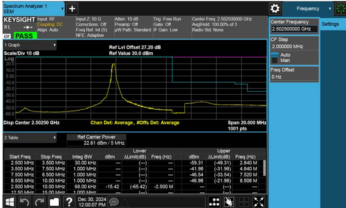
Sub6 n7. Low Channel Edge Plot (5 MHz Ch.500500 BPSK_RB 1)-2
