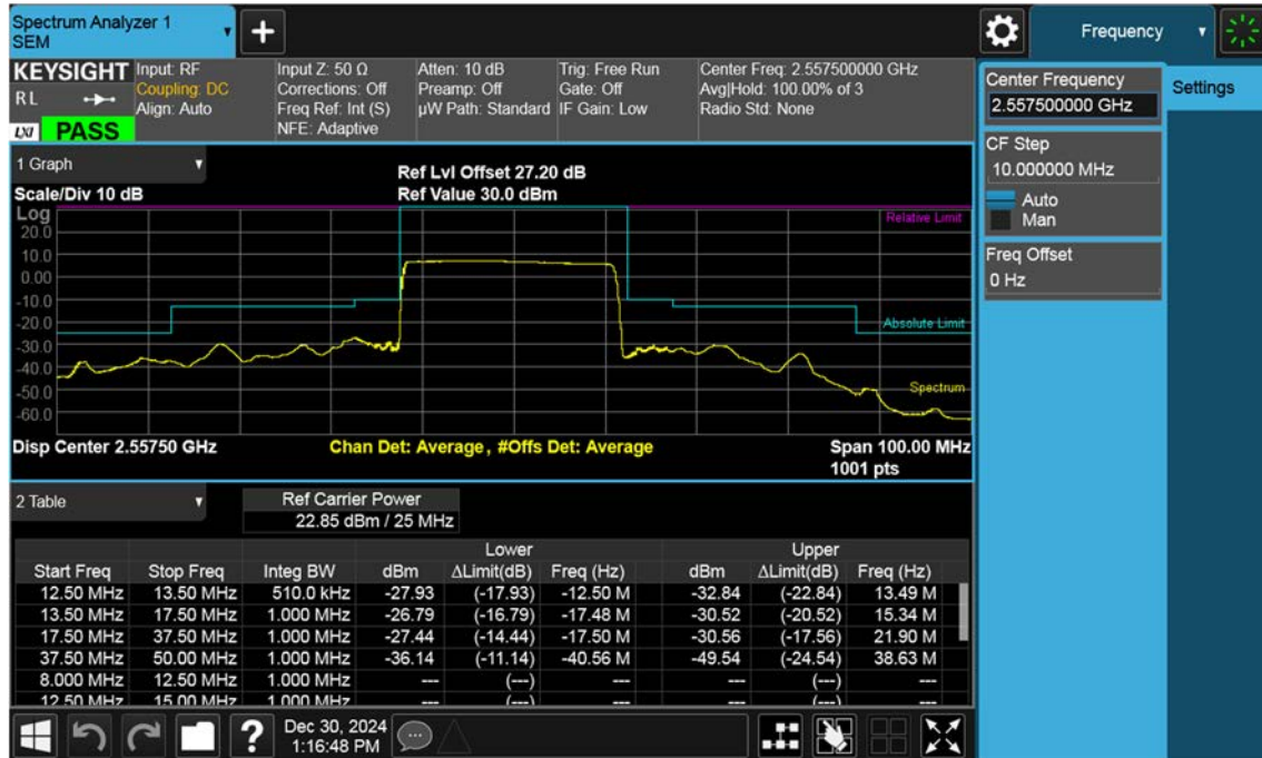
Sub6 n7. High Channel Edge Plot (25 MHz Ch.511500 BPSK)
