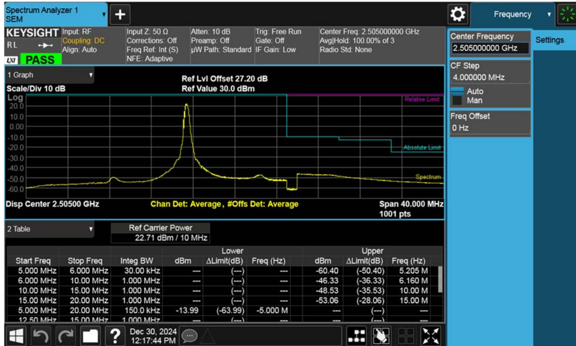
Sub6 n7. Low Channel Edge Plot (10 MHz Ch.501000 BPSK RB 1)-2
