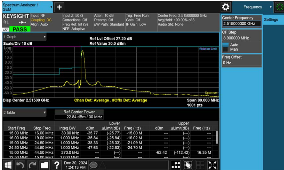
Sub6 n7. Low Channel Edge Plot (30 MHz Ch.503000 BPSK RB 1)-1
