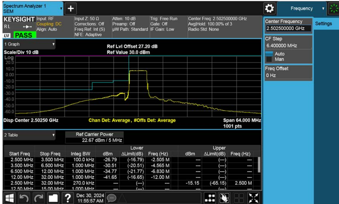
Sub6 n7. Low Channel Edge Plot (5 MHz Ch.500500 BPSK)-1
