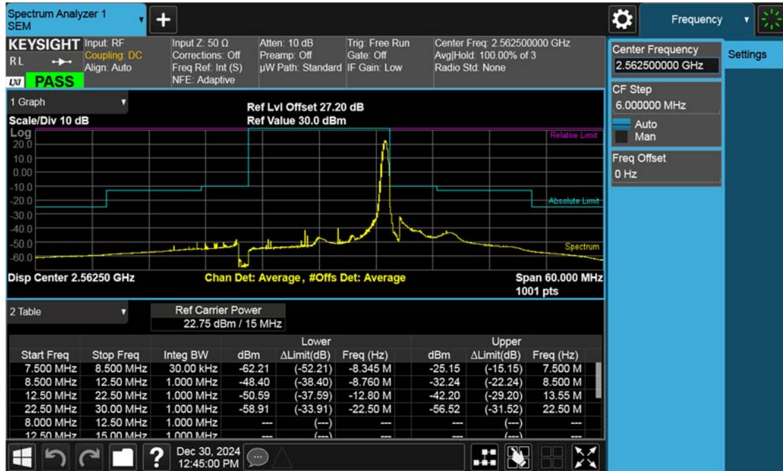
Sub6 n7. High Channel Edge Plot (15 MHz Ch.512500 BPSK RB 1)
