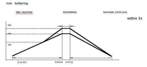
Recommended temperature profiles for re-flow soldering in Figure 1.
