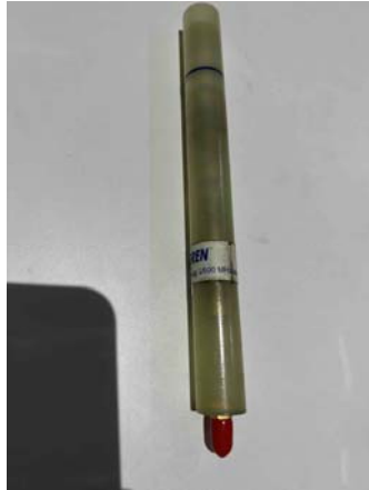
Fig 2 dipole model 3126-2500 frequency 2500 MHz
