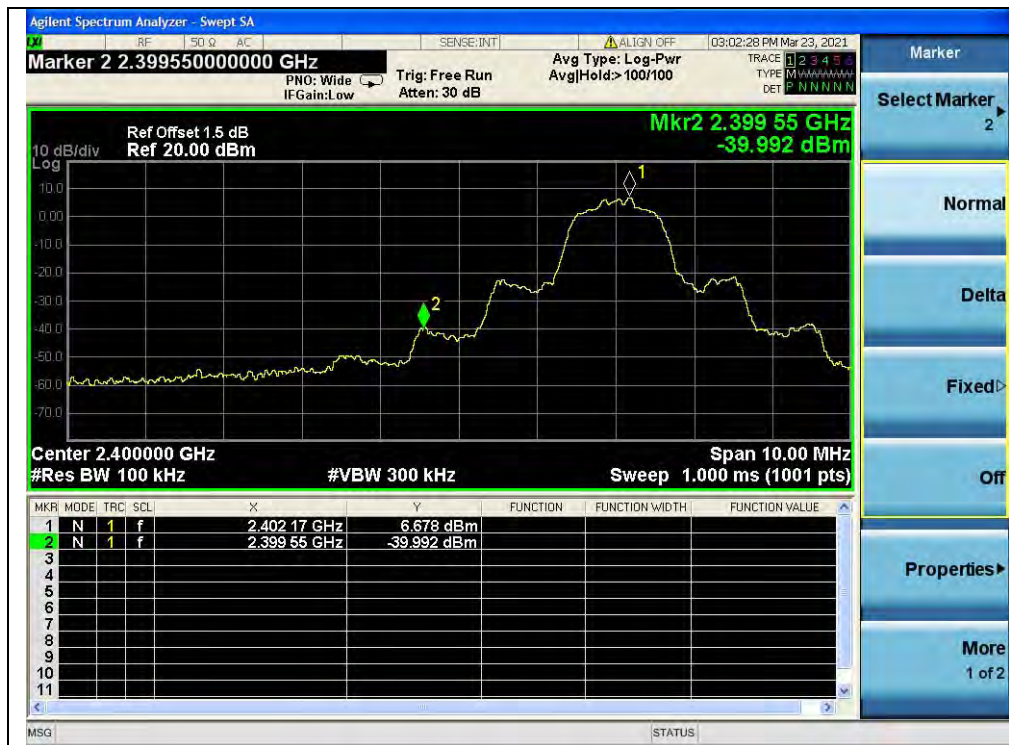
(Band edge, Channel 0, \pi/4 -DQPSK)
