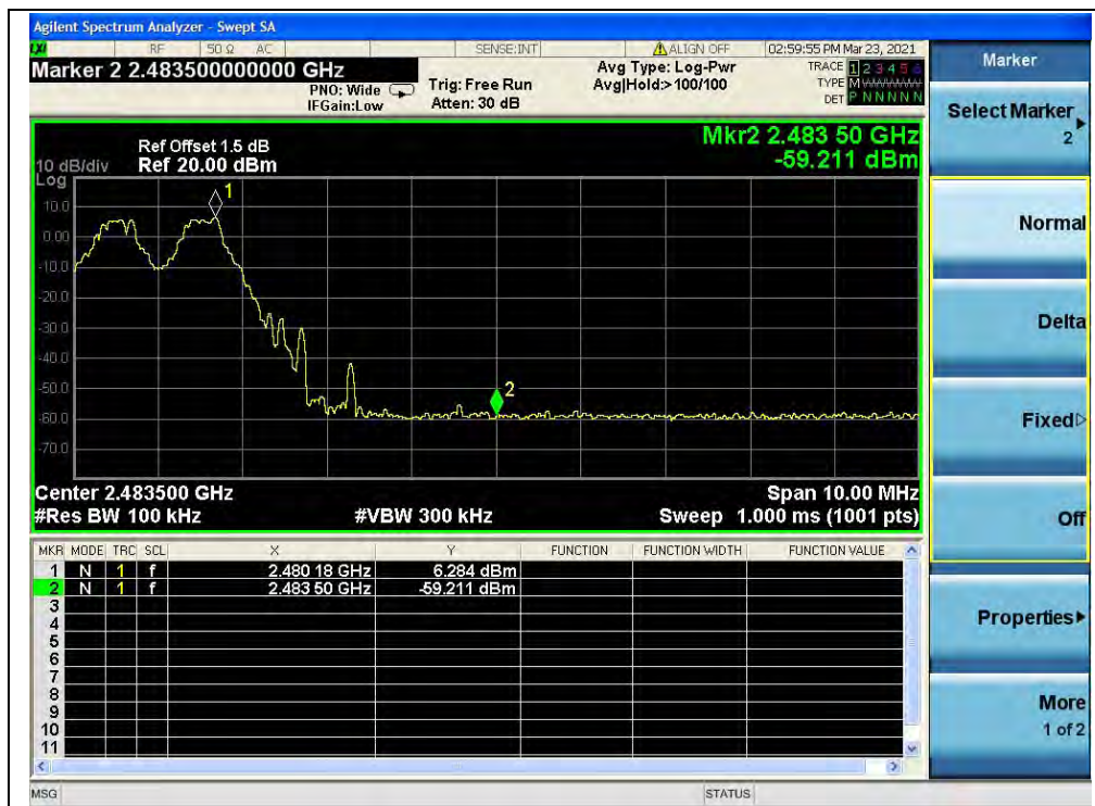
(Band edge with hopping on, Channel 78, GFSK)
