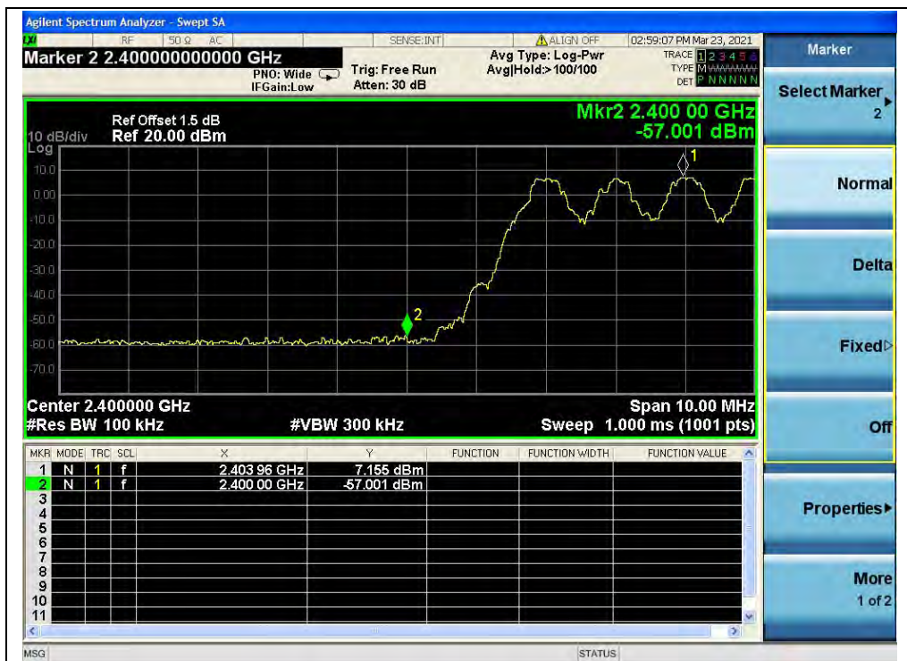
(Band edge with hopping on, Channel 0, GFSK)
