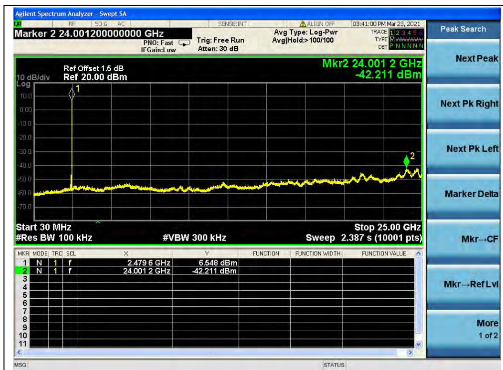
(30MHz to 25GHz, Channel 78, GFSK)
