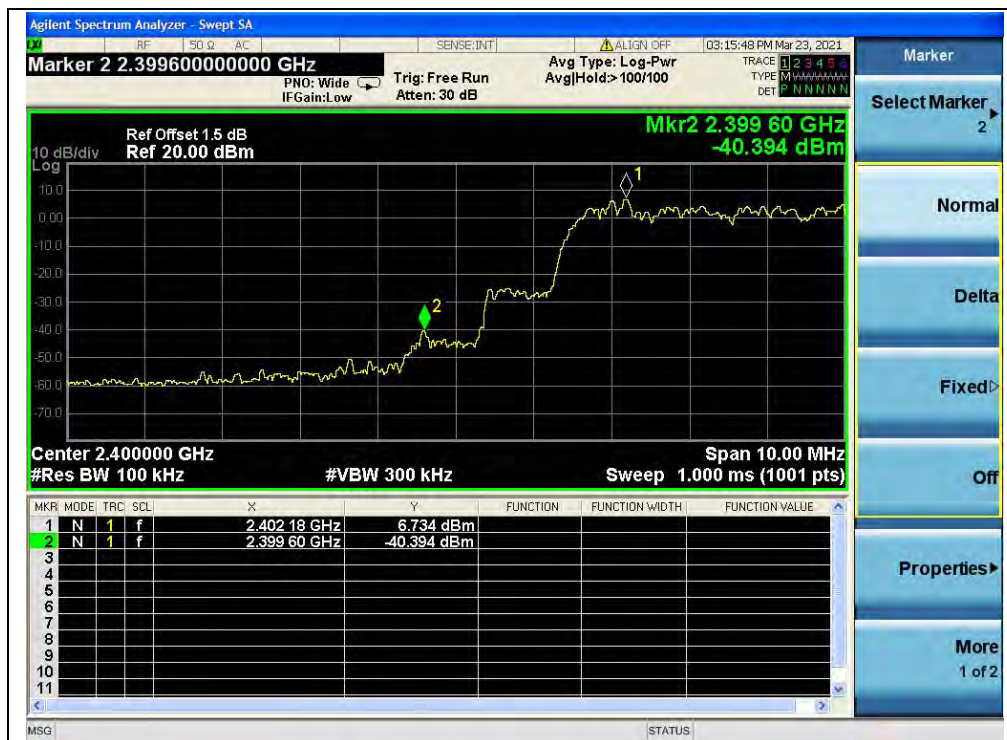
(Band edge with hopping on, Channel 0, 8-DPSK)
