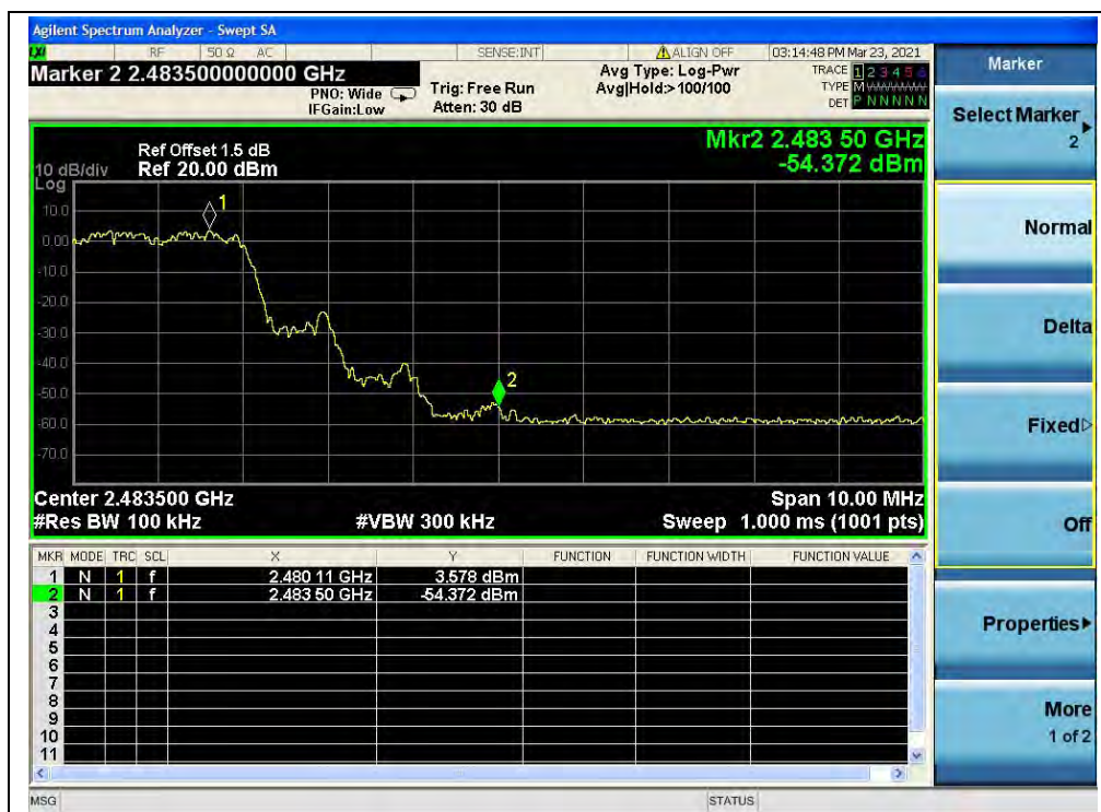
(Band edge with hopping on, Channel 78, 8-DPSK)
