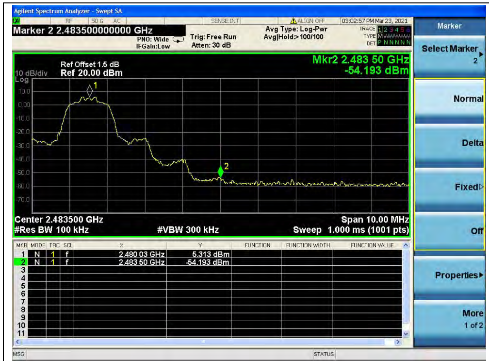
(Band edge, Channel 78, \pi/4 -DQPSK)
