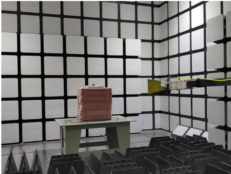
Radiated Emissions View (Above 1 GHz)
