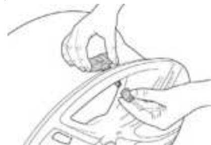
Screw the nut onto the sensor valve by hand.
