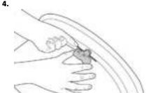
Place the anti-rotation pin into the valve hole to prevent movement of the sensor during tightening.
