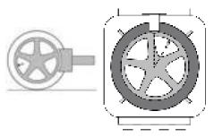
Break the bead of the tire ensuring the valve is located on Place the valve through the valve hole, ensuring the rubber When the tire is dismounted the valve must be located at 1 o'clock to the tire fitting head.
