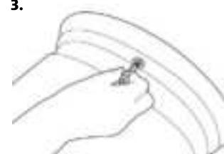
Place the valve stem through the valve hole, ensuring the rubber makes good contact with the valve hole all around.
