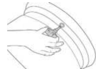
Break the bead of the tire ensuring the valve is located on the opposite side of the rim from the bead breaker blade. When the tire is dismounted the valve must be located at 1 o'clock to the tire fitting head.
