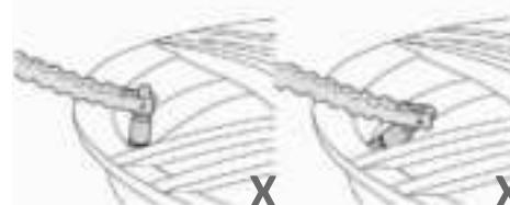
Please note: failure to pull the valve through at the correct angle can result in damage to the valve stem or prevent the rubber from creating an air-tight seal.
