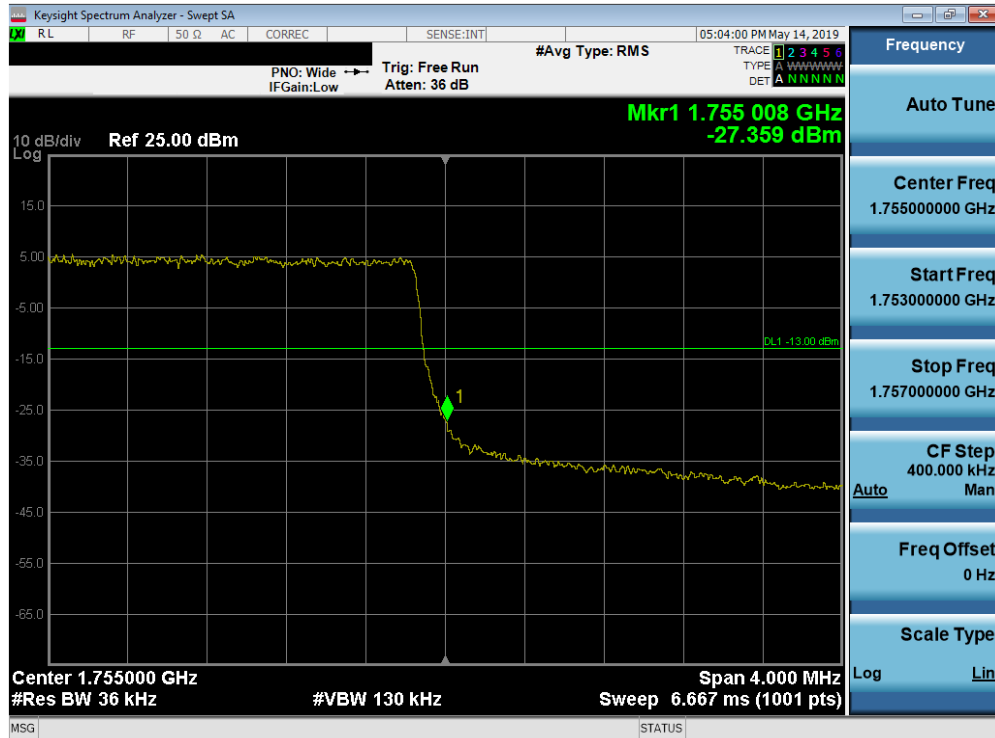
Plot 7-203. Upper Band Edge Plot (Band 4 - 3.0MHz QPSK - Full RB Configuration)
