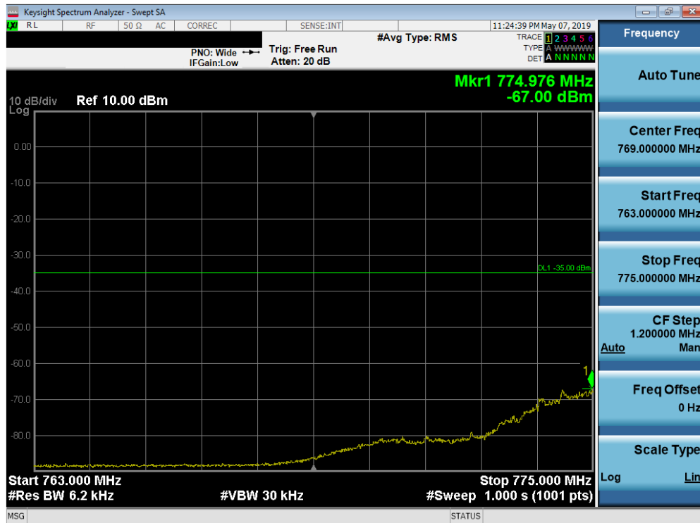
Plot 7-178. Lower Emission Mask Plot (Band 13 - 5.0MHz QPSK - Full RB Configuration)
