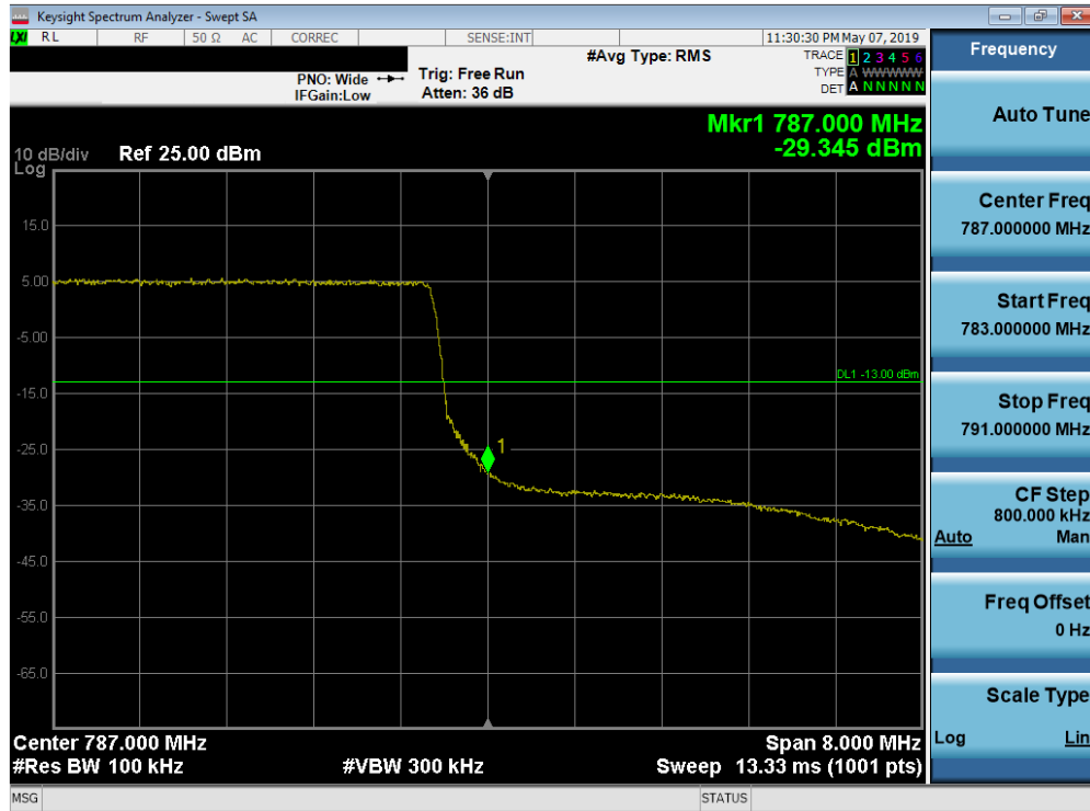
Plot 7-183. Upper Band Edge Plot (Band 13 - 10.0MHz QPSK - Full RB Configuration)
