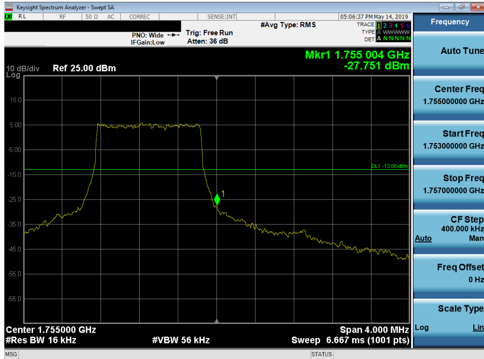
Plot 7-197. Upper Band Edge Plot (Band 4 - 1.4MHz QPSK - Full RB Configuration)
