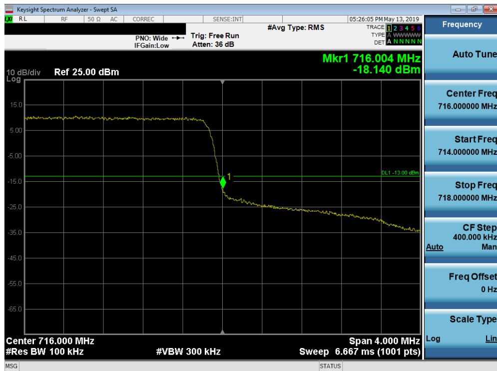
Plot 7-168. Upper Band Edge Plot (Band 12 - 3.0MHz QPSK - Full RB Configuration)
