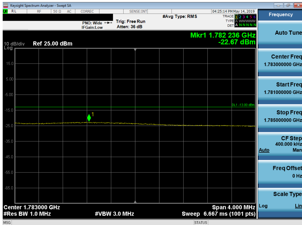
Plot 7-224. Upper Extended Band Edge Plot (Band 66 - 15.0MHz QPSK - Full RB Configuration)
