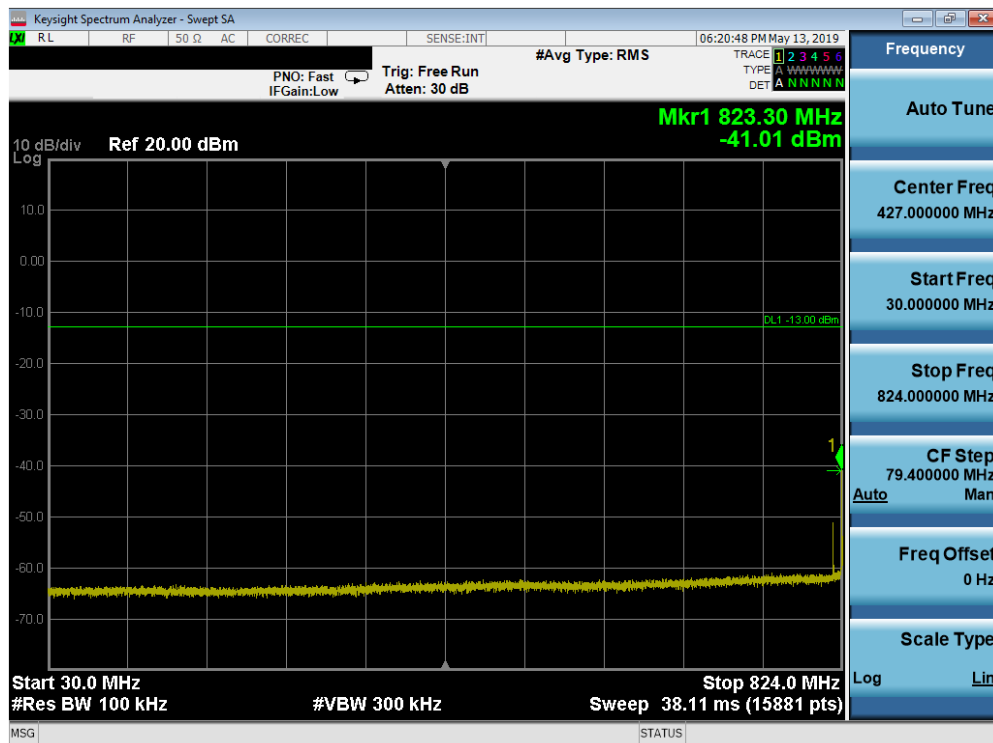
Plot 7-124. Conducted Spurious Plot (Band 26/5 - 10.0MHz QPSK - RB Size 1, RB Offset 0 - Mid Channel)
