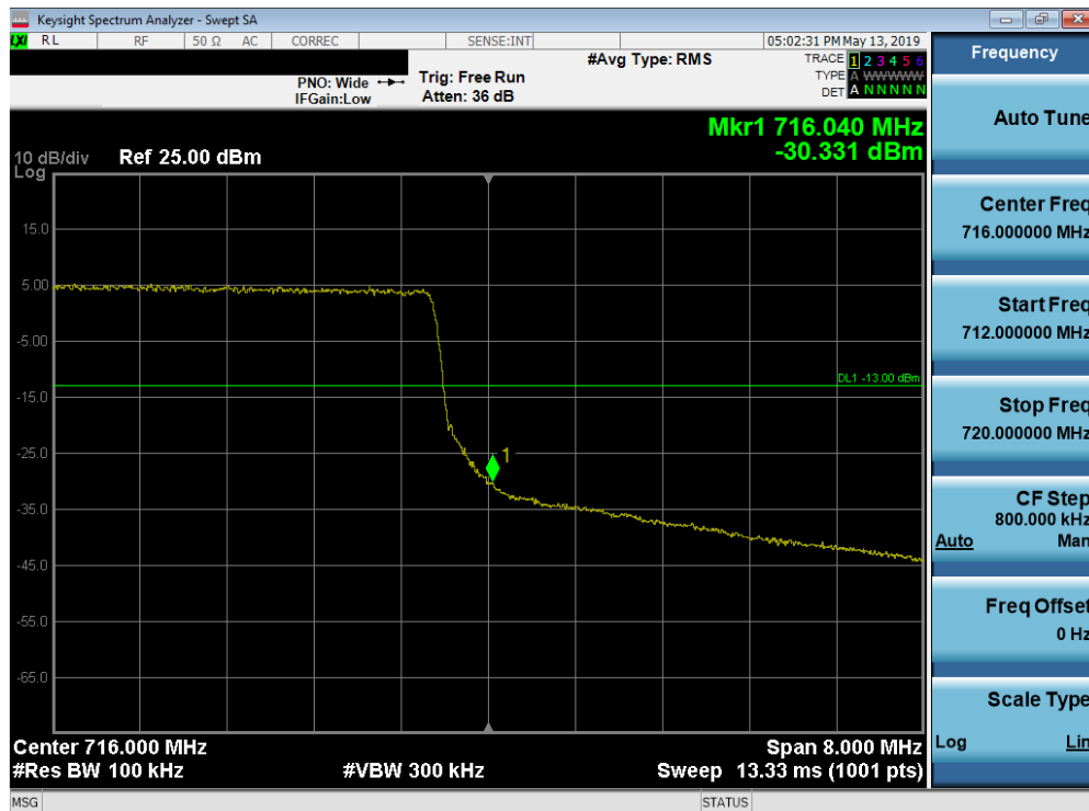
Plot 7-176. Upper Band Edge Plot (Band 12/17 - 10.0MHz QPSK - Full RB Configuration)
