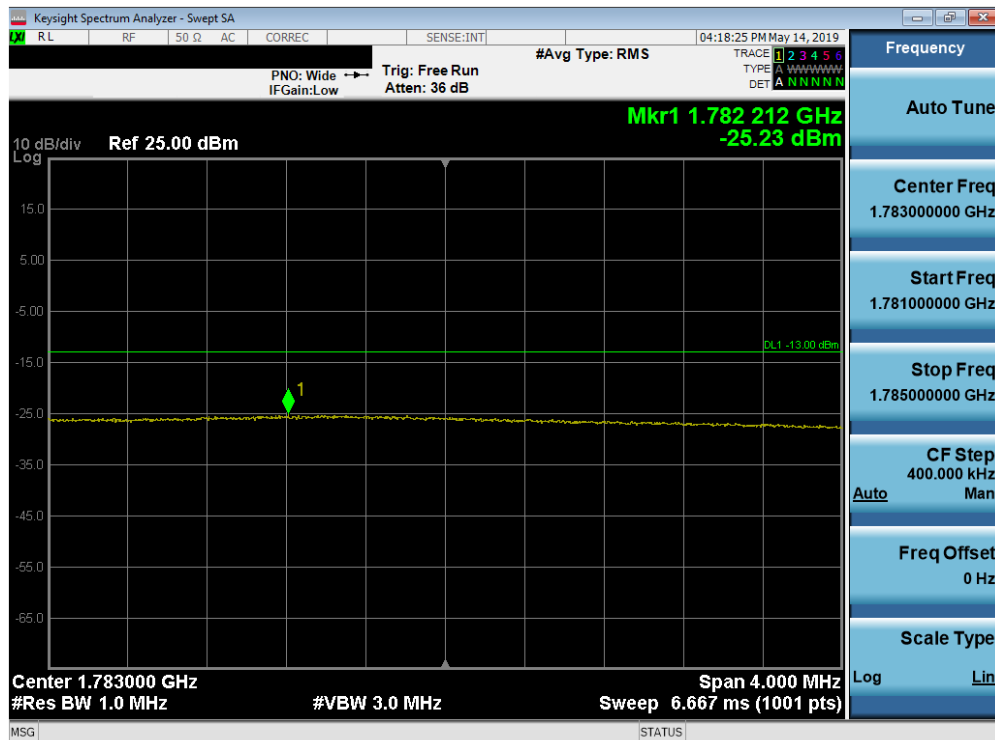
Plot 7-230. Upper Extended Band Edge Plot (Band 66 - 20.0MHz QPSK - Full RB Configuration)
