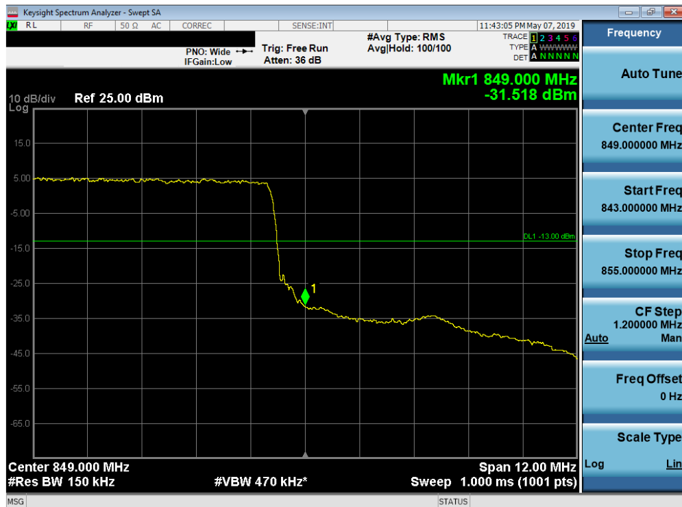
Plot 7-194. Upper Band Edge Plot (Band 26 - 15.0MHz QPSK - Full RB Configuration)
