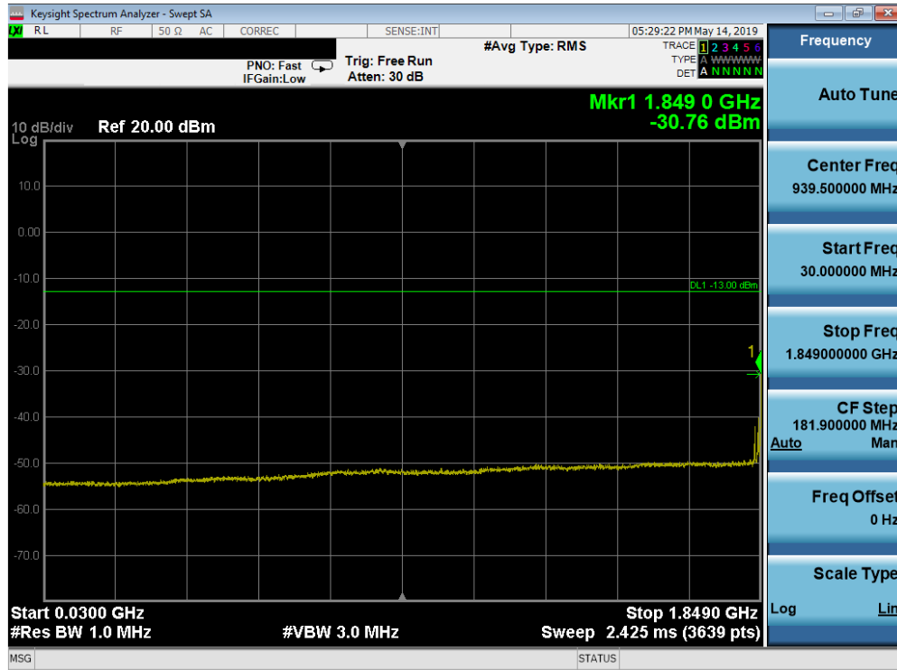
Plot 7-139. Conducted Spurious Plot (Band 25/2 - 20.0MHz QPSK - RB Size 1, RB Offset 0 - Low Channel)
