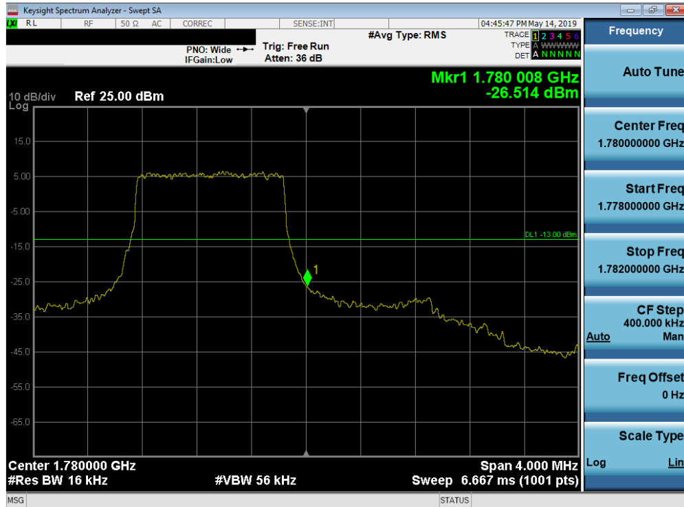
Plot 7-199. Upper Band Edge Plot (Band 66 - 1.4MHz QPSK - Full RB Configuration)
