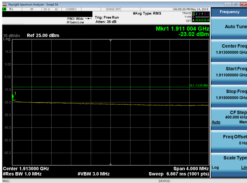
Plot 7-252. Upper Extended Band Edge Plot (Band 2 - 10.0MHz QPSK - Full RB Configuration)
