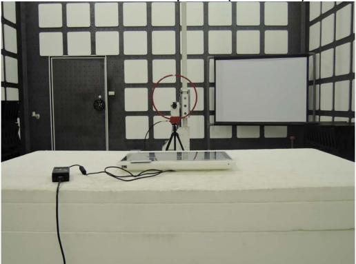
Radiated Emission Setup Photos (Below 1GHz)
