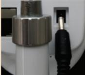
Connect the power adapter to the camera power socket.
