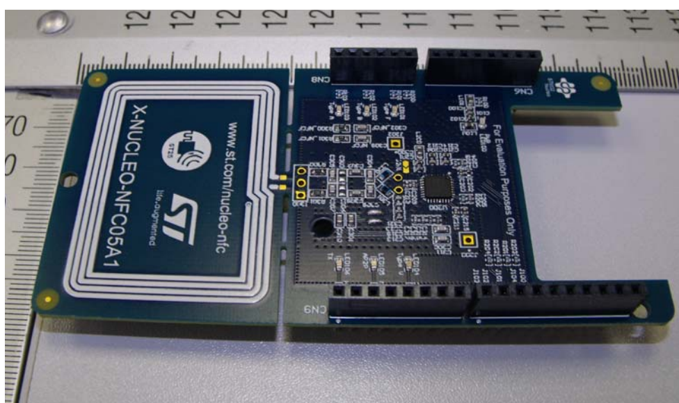
Figure 2: X-NUCLEO-NFC05A1 – Top side
