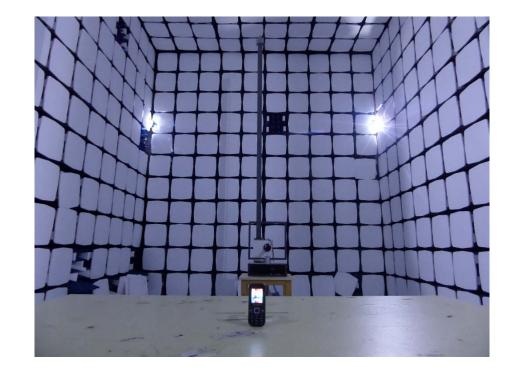
Spurious Radiation Test Setup (9kHz to 30MHz)
