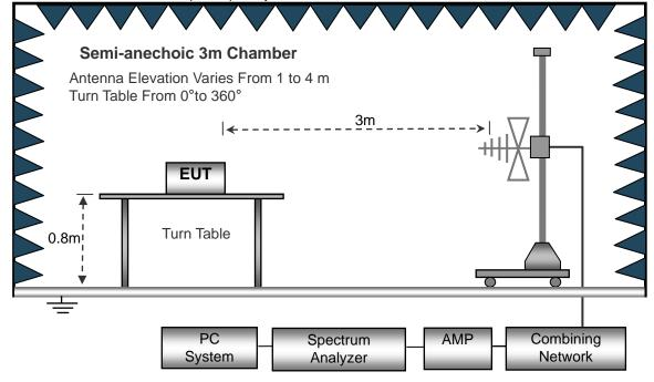
(C) Radiated Emission Test-Up Frequency Above 1GHz
