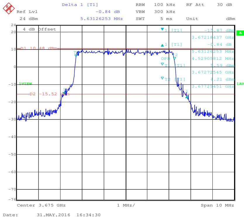
**QPSK (10MHz), Middle Channel**
