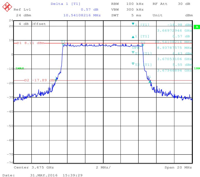
**QPSK (15MHz), Middle Channel**
