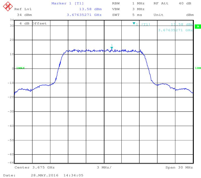
**QPSK (15MHz), High Channel**
