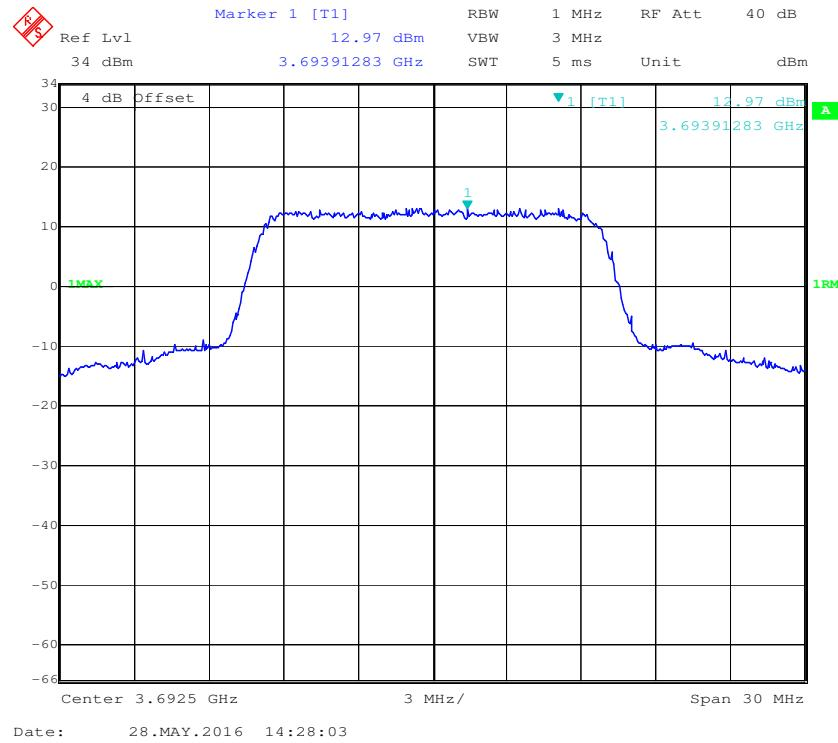
**QPSK (20MHz), Low Channel**
