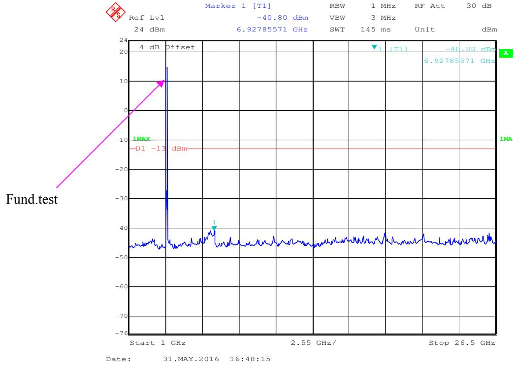
**16QAM(15M)(Channel 1 GHz-26.5 GHz)**
