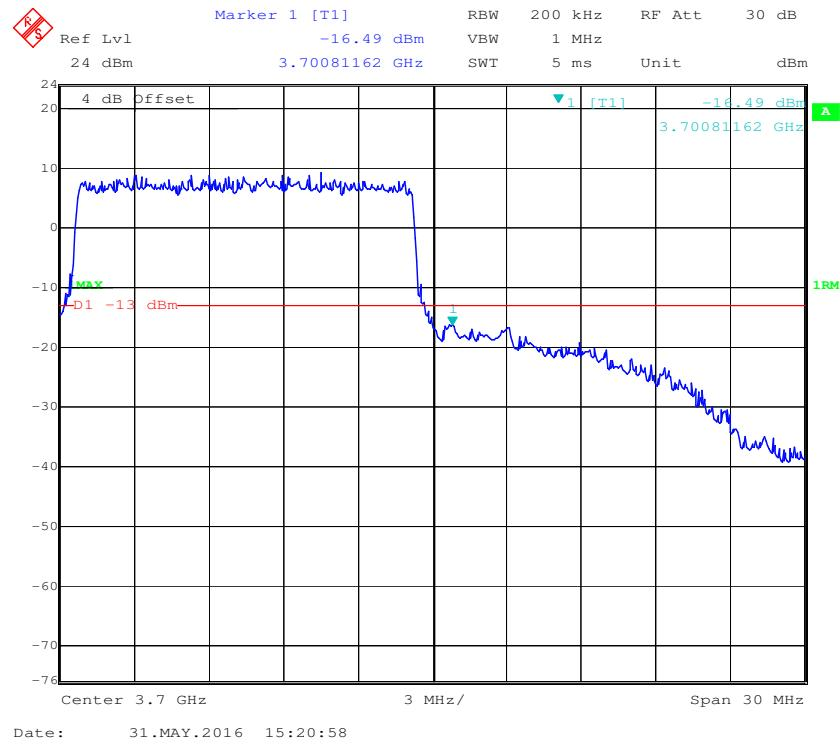
**QPSK (20MHz), Left Side**
