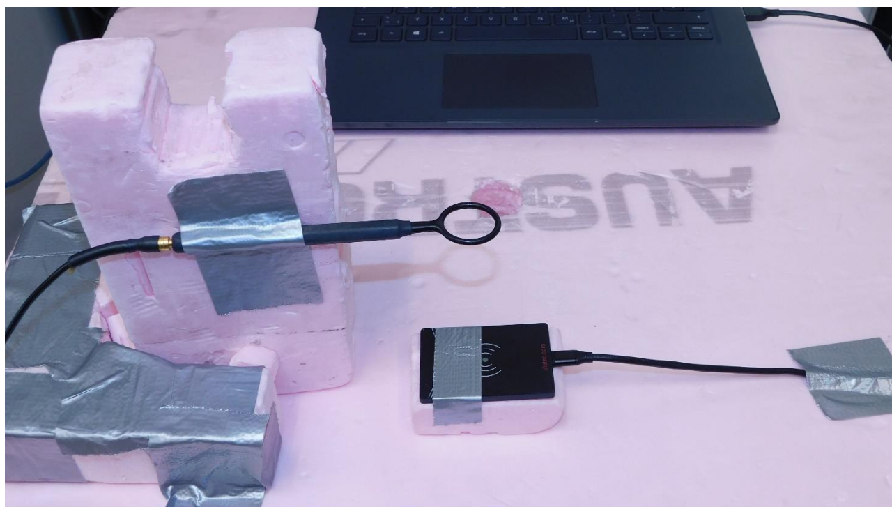
Picture 9: Test setup-Occupied bandwidth tests
