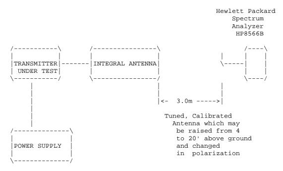
Method of Measuring Radiated Spurious Emissions
