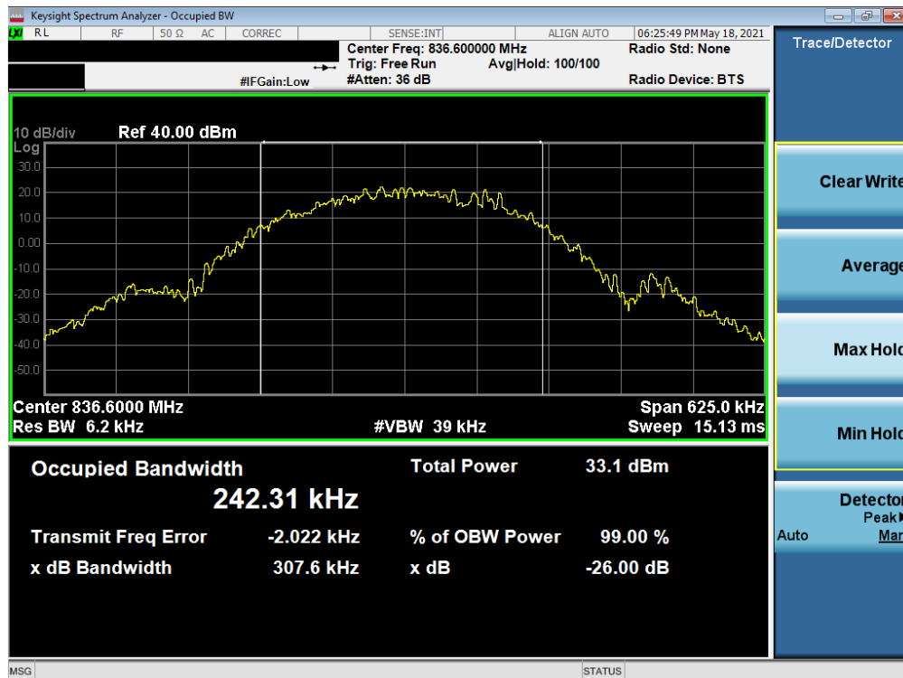
Plot 7-12. Occupied Bandwidth Plot (EDGE, Ch. 190)
