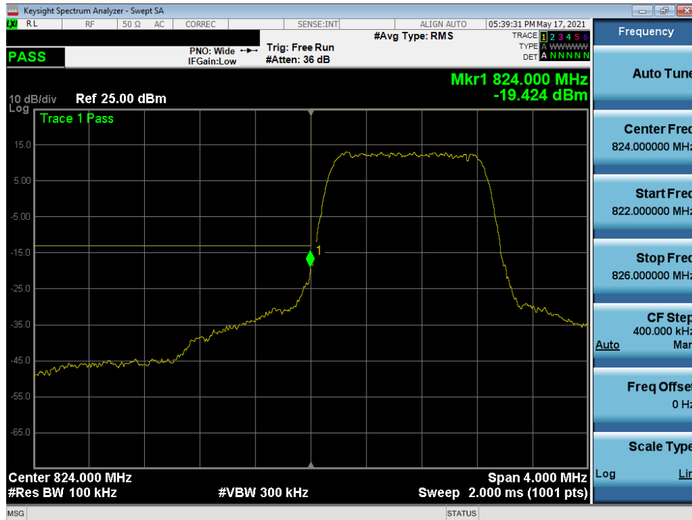
Plot 7-49. Lower Band Edge Plot (LTE Band 26/5 – 1.4MHz QPSK – Full RB)
