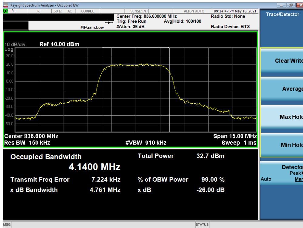
Plot 7-13. Occupied Bandwidth Plot (WCDMA, Ch. 4183)
