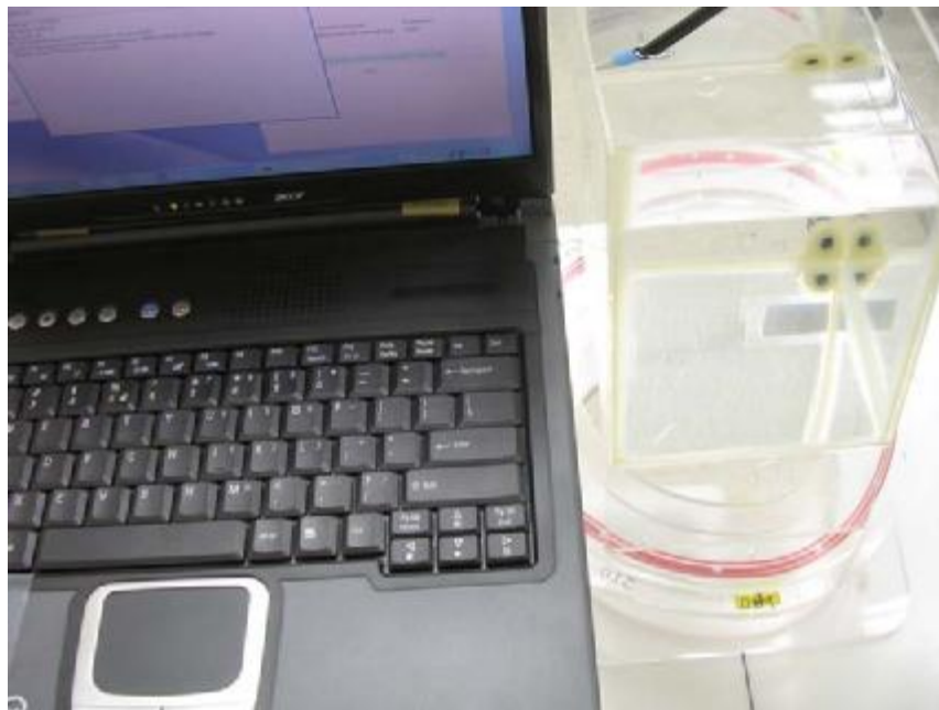
EUT right to the phantom, 15 mm separation
