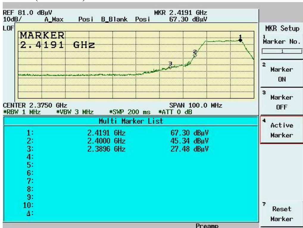
**Band Edge measurement for radiated emission in Restricted Band(Radiated) Average Mode (Channel 1)**
