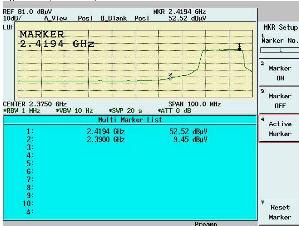
**Band Edge measurement for radiated emission in Restricted Band(Radiated) Peak Mode (Channel 11)**
