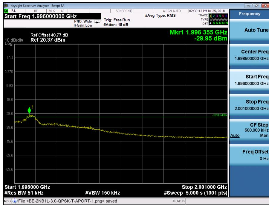
The channel power of 1MHz for 1996.355MHz is -21.66dBm, which is within the limit of -19.02dBm
