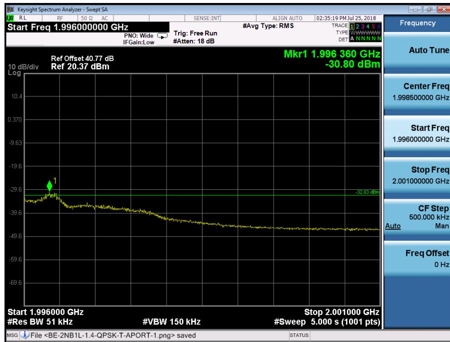
The channel power of 1MHz for 1996.360MHz is -21.32dBm, which is within the limit of -19.02dBm
