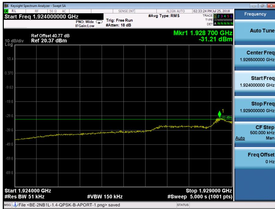
The channel power of 1MHz for 1928.700MHz is -20.93dBm, which is within the limit of -19.02dBm
