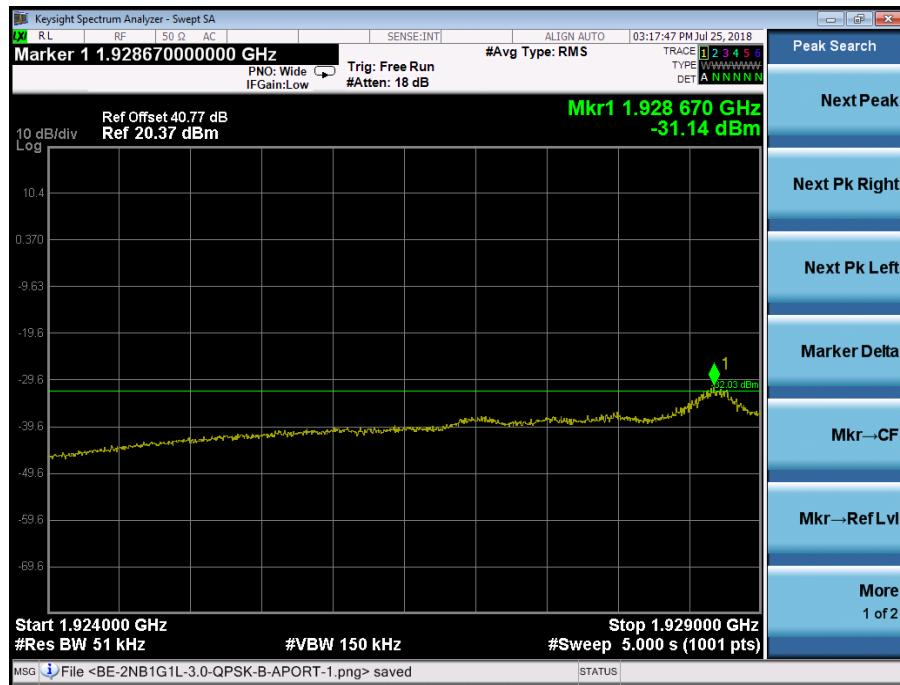
The channel power of 1MHz for 1928.670MHz is -22.23dBm, which is within the limit of -19.02dBm
