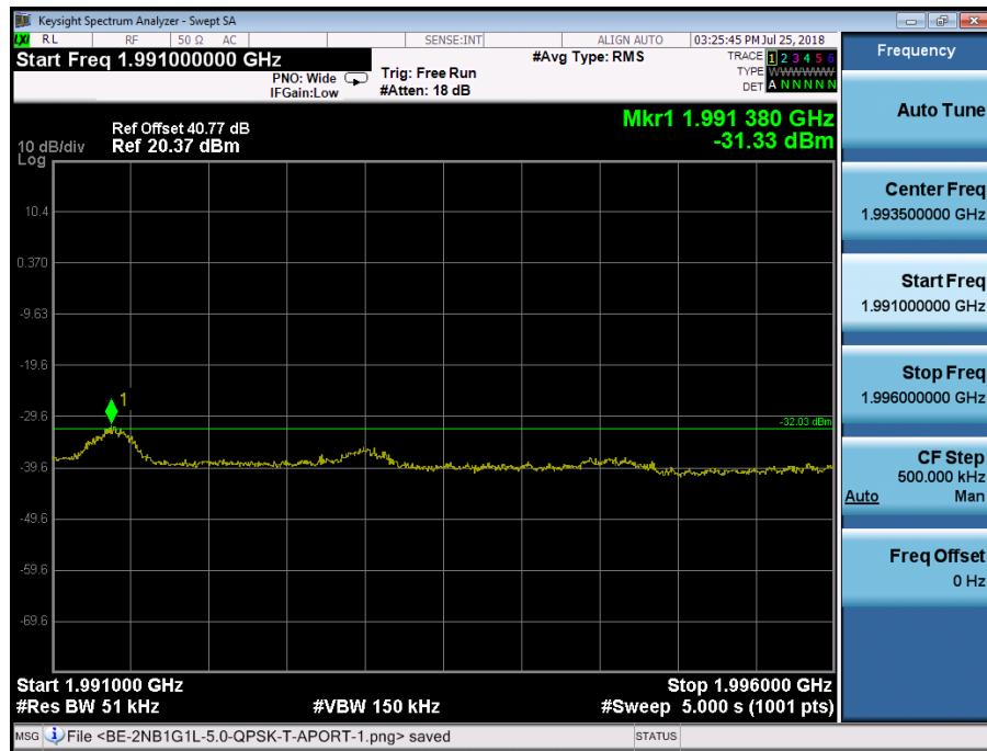
The channel power of 1MHz for 1991.380MHz is -23.01dBm, which is within the limit of -19.02dBm
