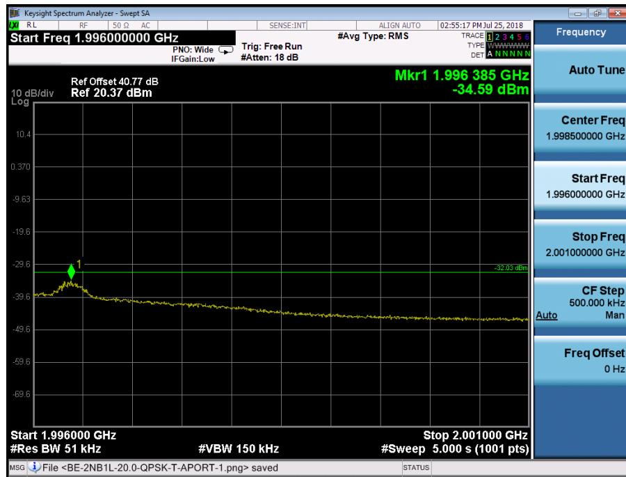
Configuration NB-IoT-IB+LTE -MIMO-MC-1-BE, (1IB, QPSK +1LTE, QPSK)
