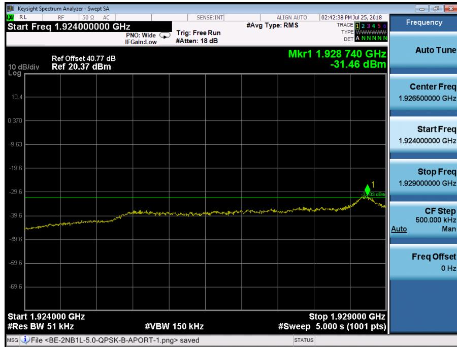
The channel power of 1MHz for 1928.740MHz is -21.67dBm, which is within the limit of -19.02dBm
