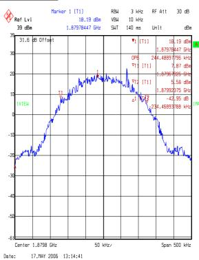
Note: The occupied bandwidth is measured using the internal OBW function of the measurement analyser. The analyser automatically configures the measurement bandwidths to make an accurate measurement.
