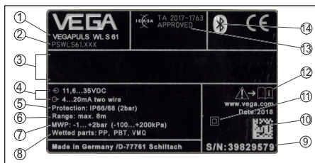
Abb. 17: Layout of the type label (example)
