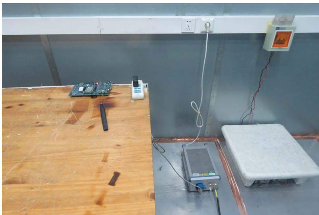
Picture 2 Conducted Emission Test Setup
