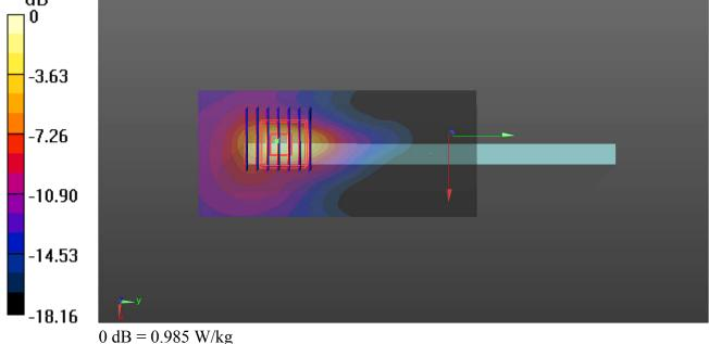
Communication System: UID 0, WIFI (0); Frequency: 2412 MHz; Duty Cycle: 1:1.013
