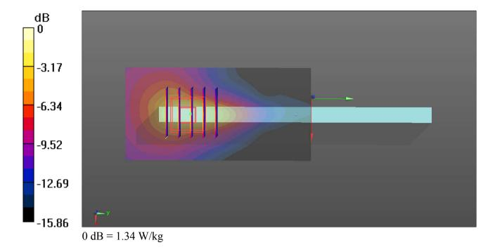
Communication System: UID 0, UMTS (0); Frequency: 1852.4 MHz; Duty Cycle: 1:1
