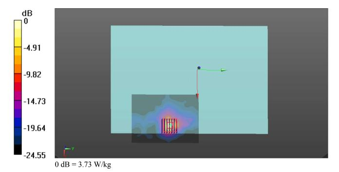
Communication System: UID 0, WIFI (0); Frequency: 5260 MHz; Duty Cycle: 1:1.066 Medium: MSL\_5250\_160805 Medium parameters used: f = 5260 MHz;  $\sigma$  = 5.429 S/m;  $\epsilon_r$  = 48.444;  $\rho$
