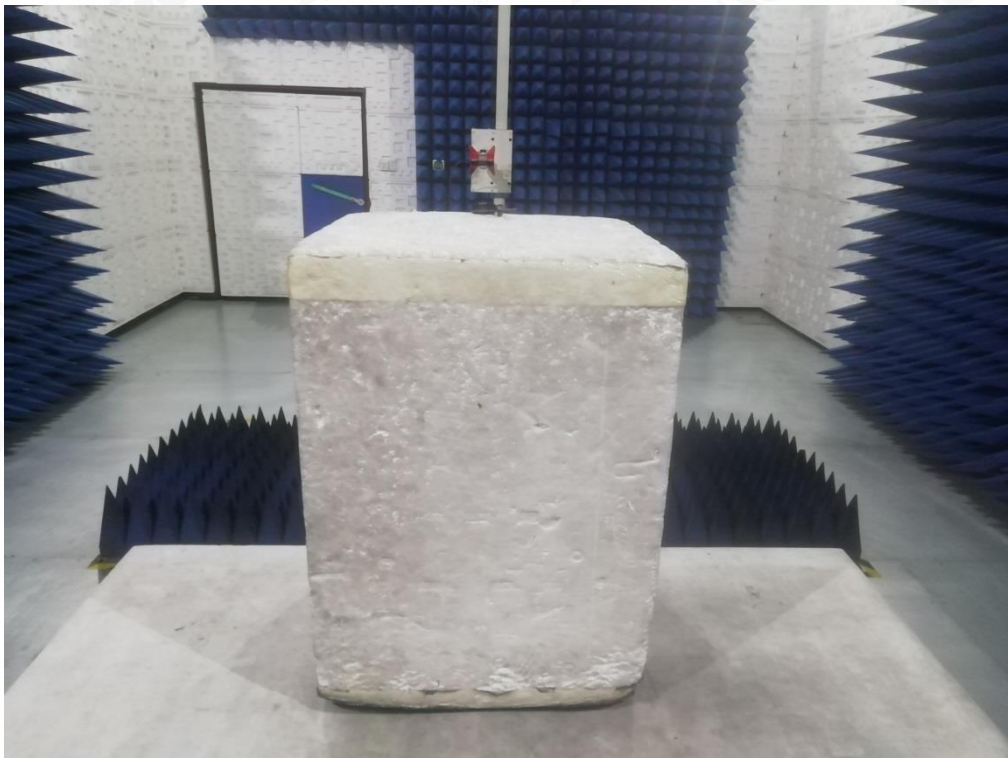
RADIATED EMISSION ABOVE 1G TEST SETUP
