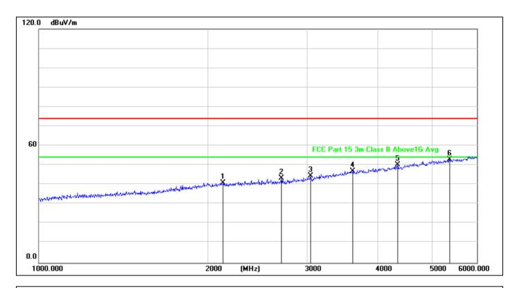
Site: LAB Antenna::Horizontal Temperature(C):26(C)
