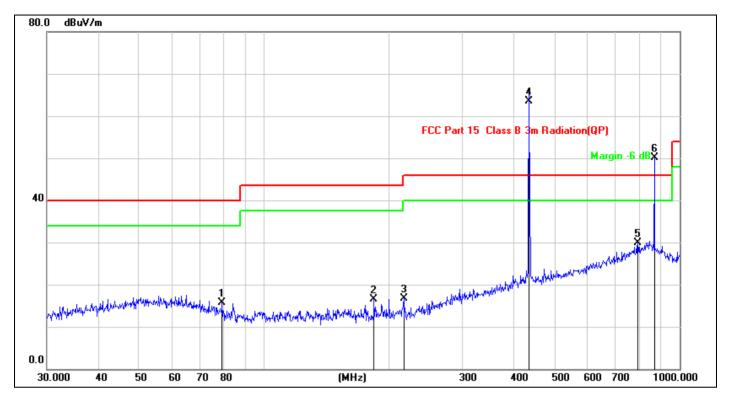
Site: LAB Antenna:: Vertical Temperature(C):26(C) FCC Part 15 C 3m Radiation **Humidity(%):54%** Limit: **EUT: Test Time:** 2023/03/02 9:06:34 **RF Remote Controller Power Rating:** DC 3V M/N.: AS-2301 Mode: TX **Test Engineer:** Sunshine Note:
