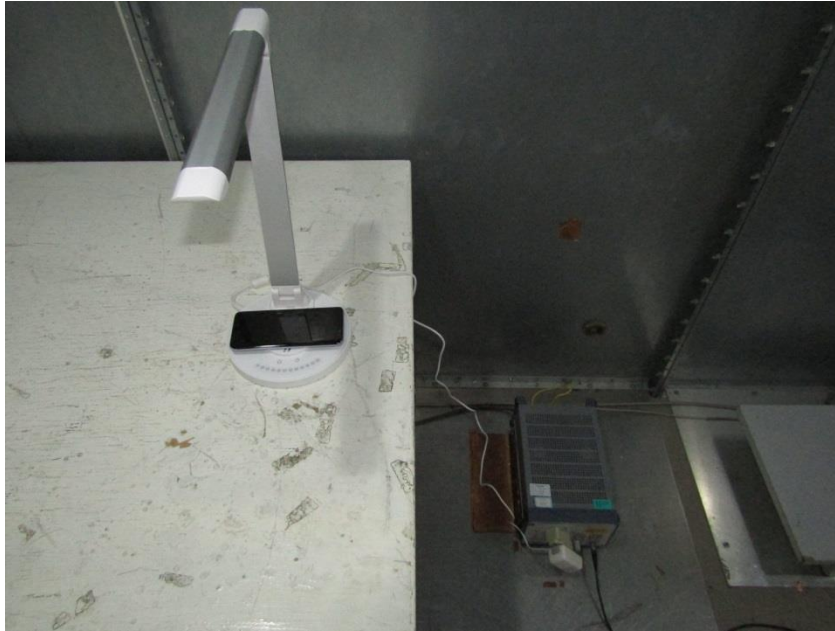
Measurement of Conducted Emission Test Set Up
