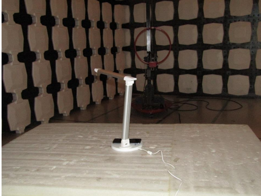
Measurement of Radiated Emission Test Set Up
