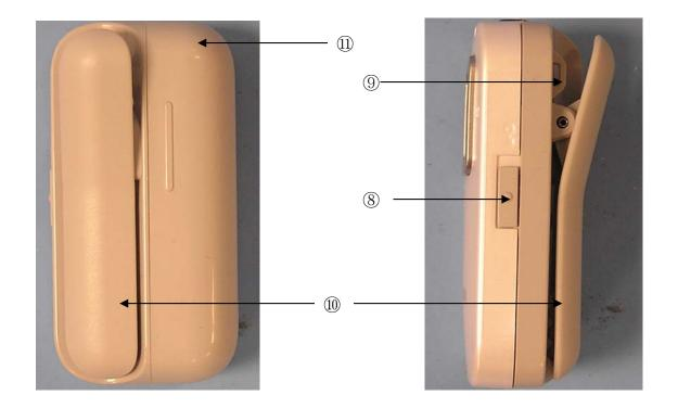
**8 Hold switch:** Press to deactivate the buttons of the main unit to prevent misoperation. Release before operation to activate the buttons.
