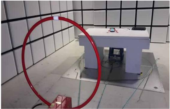
Radiated Emission Set up Photos (Below 1GHz)
