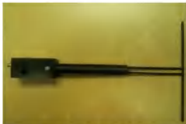
Figure 1 – MVG COMOSAR Validation Dipole
