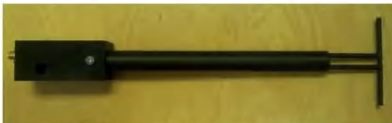
Figure 1 – MVG COMOSAR Validation Dipole
