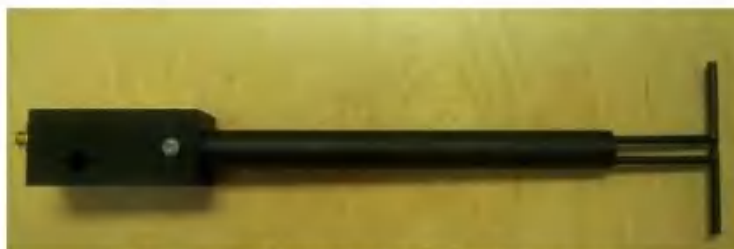
Figure 1 – MVG COMOSAR Validation Dipole
