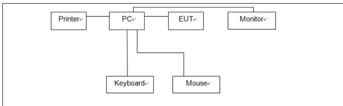
**3.5. Support unit used in test configuration**
