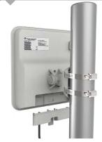
Remove cap and connect RJ 45 cable to the radio.
