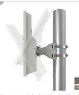
Align radio to required angle by tilting up and down. The maximum radio tilting angle is ± 40°, with an incremental of 10°. Secure radio with max 5.0 Nm torque.
