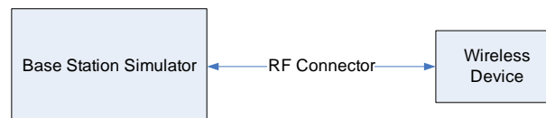
Figure 9-4 Power Measurement Setup
