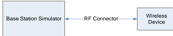
Figure 9-2 Power Measurement Setup
