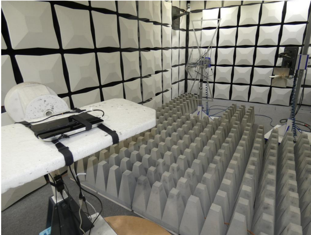
Photo 3: Test setup for radiated measurements above 1 GHz
